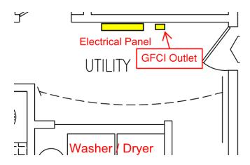
4)Push the reset button on the GFCI power outlet
